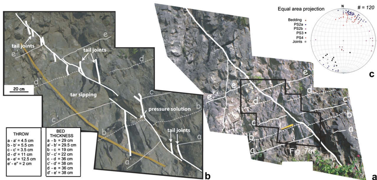
Fig. 7. (a) Normal fault with a throw up to 12.5 cm. In order to calculate the amount of offset, we distinguished five different beds, here named a–e, respectively. The dotted line represents the location of Fig. 7(b). (b) Close-up of the fault. Several isolated slip surfaces are present along the fault, around which tail joints are present at their extensional quadrants and in correspondence of the releasing jogs. Conversely, tail pressure solution seams are present within contractional jogs. The bedding thickness on the two sides of the fault is reported in the lower table, which also shows the amount of vertical offset measured along the individual slip surfaces. (c) Lower hemisphere equal area projection of the poles relative to the different structural elements measured along this fault.
